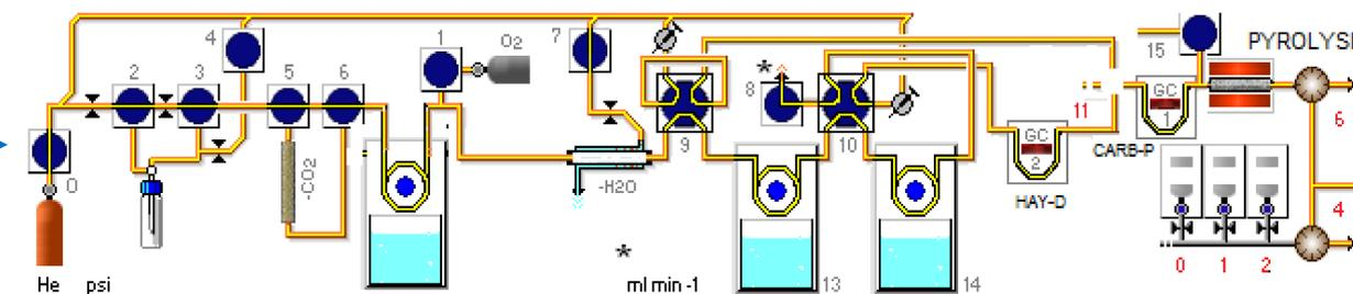
**Figure 2:** Schematics of the CryoGas system in both carbon (top) and hydrogen (bottom) modes. Showing a series of chemical and cryo traps as well as the configuration of GC columns/ vents for the separation of  $\text{CH}_4$  from air components.
