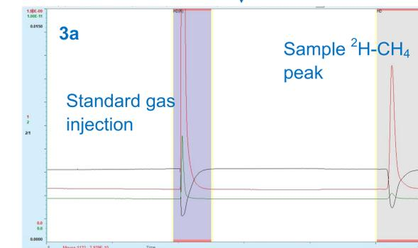
**Figure 3a)** A typical  $\delta^2\text{H}$  - $\text{CH}_4$  in air output, with initial ref gas pulse followed by a  $>1$  nano amp sample peak height.
