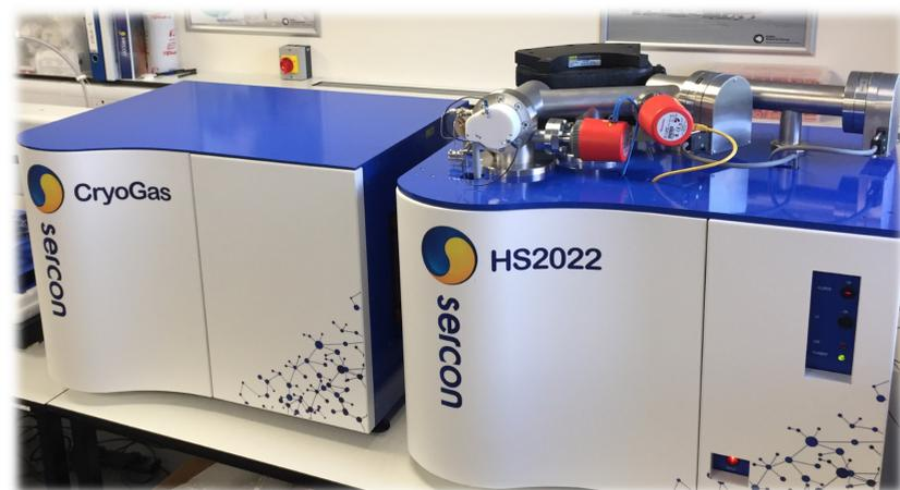
**Figure 1:** The Sercon CryoGas and HS2022 mass spectrometer, this is the first Sercon instrument built specifically for the analysis of C and H in methane.
